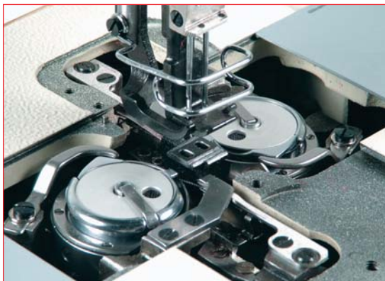
Thread trimming device and large hooks.
