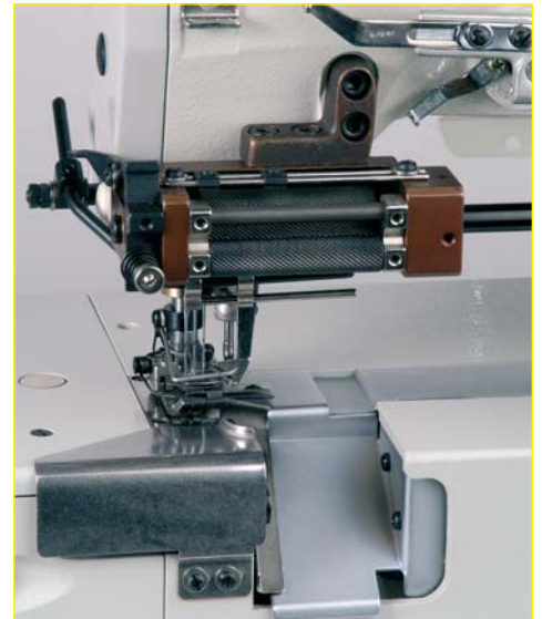
Top metering device on Global® FB 2553-64 TMD
