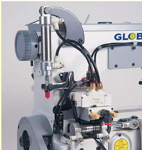
Pneumatic thread trimmer and presser foot lift
