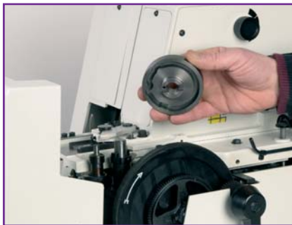
The cams of the BH 1000 are easily interchangeable; just remove and replace
