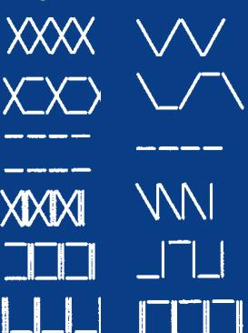
**OS 7200 – Ornamental stitch, cylinderbed machine with 2 needles, which can carry out functional and ornamental stitching on uppers, suitcases, bags etc. 12 different patterns by interchangeable cams.**
