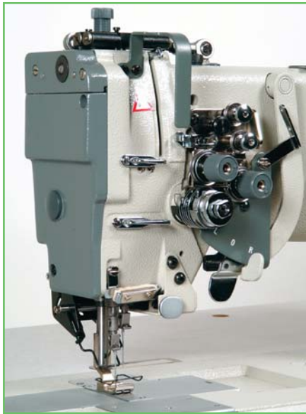
Disengageable needle bars.
